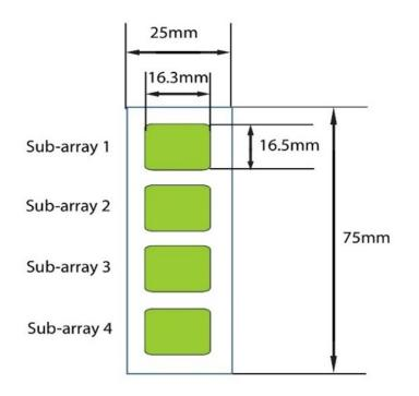
Four identical sub-arrays on one slide
