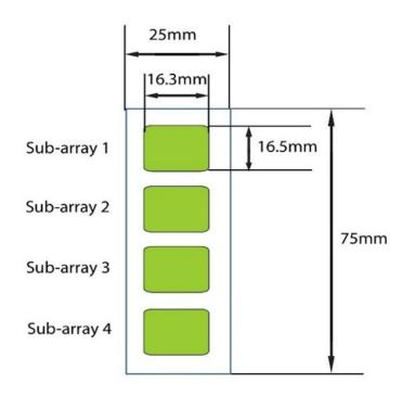
Four identical sub-arrays on one slide
