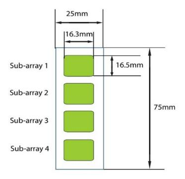
4 printed sub-arrays per glass chip
