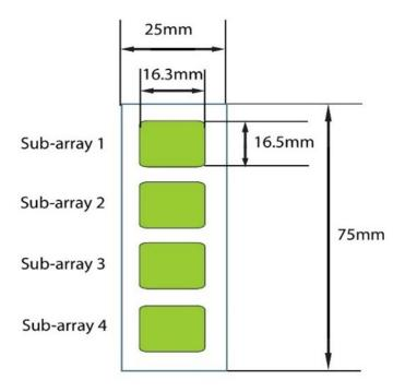
4 printed sub-arrays per glass chip
