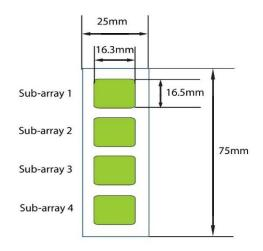
4 printed sub-arrays per glass chip
