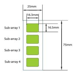
4 printed sub-arrays per glass chip
