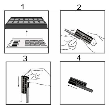
Note: You may assemble and disassemble the glass slide into an incubation chamber and glass slide using the following steps.
