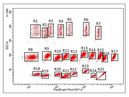
**Figure 2. Different populations of bead size and color combinations ("R#") enable multiplex protein detection with RayPlex arrays.** *Bead ID* R1 - R7: Large Beads. *Bead ID* R8 - R17: Medium Beads. *Bead ID* R18 - R25: Small Beads.
